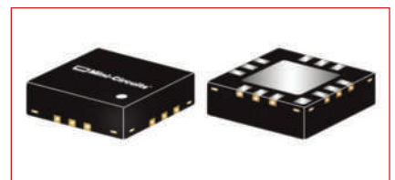
Fig. 8 Transformer fabricated with MMIC technology.
