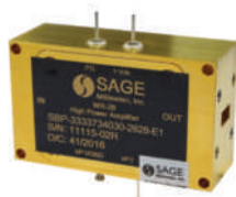
Figure 2. Dedicated Package with the Built-in Waveguide Transitions
