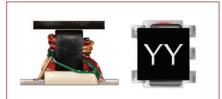
▲ Fig. 4 Construction of a wire-wound transformer with magnetic core.
